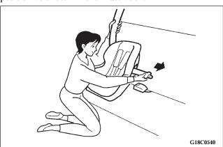
2. Route the unibelt through the child restraint system according to the child restraint system manufacturer's instructions. Then insert the unibelt latch plate into the buckle. Make sure you hear a "click" when you insert the latch plate into the buckle.
